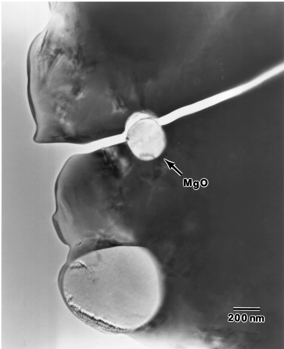
Figure 3 TEM bright field image showing microstructure of LSGM-1020, x = 0.90 , and crack propagation around a MgO inclusion.
